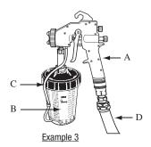
Air pressure to Spray Gun (A) is regulated and supplied to spray gun from Turbine through Air Supply Hose (D). Air pressure to the 3M<sup>TM</sup> PPS<sup>TM</sup> Type H/O Pressure Cup (B) is regulated by spray gun design and supplied through pressure port on body of spray gun to Cup Pressure Hose (C).
