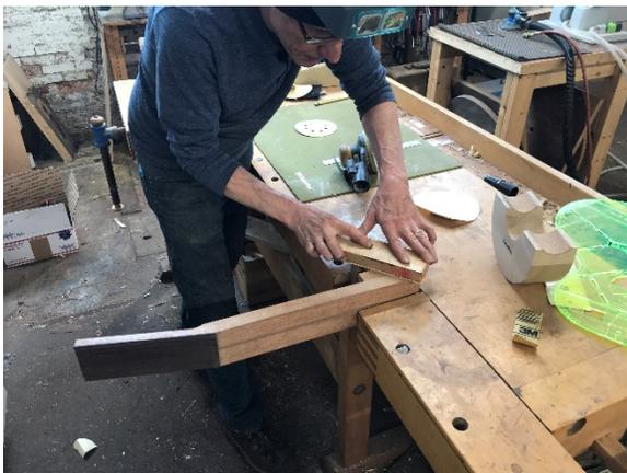
To prepare for cutting the tenon, make sure the neck blank is flush with the stacked heel.
