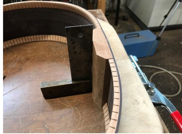
Make SURE the body is square in the mold after the screws are installed. If not put shims between the body and the mold to get it square.
