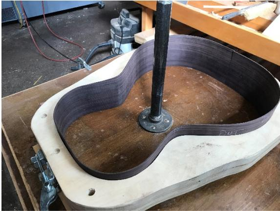
I use acrylic templates (Waldron) to lay-out the side profile and add 5mm. After bending and cutting to length, put them in the mold, top side down.
