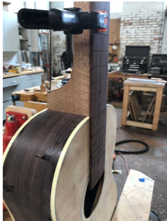
Go ahead and do the rough taper and heel sculpting. Then clamp your fingerboard to the neck and check the fit. This is the result after no flossing or tweaks!!!!
