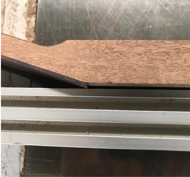
The peg head overlay keeps the blank from seating flat –
