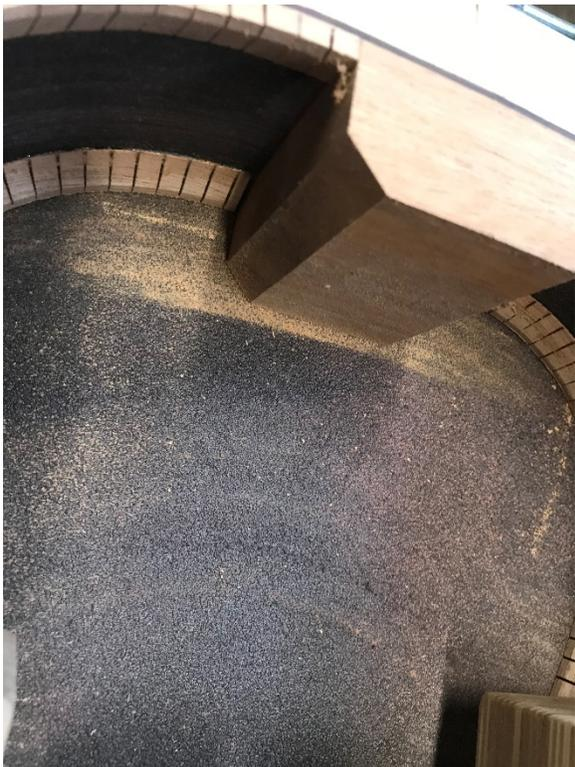
Holding the mold at the tail block end, push the neck block end and start to sand. At first you will see action at the neck block.
