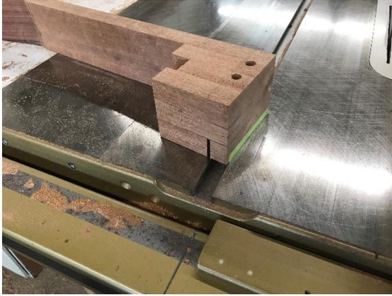
Holding the end of the heel firmly against the fence, cut one cheek.
