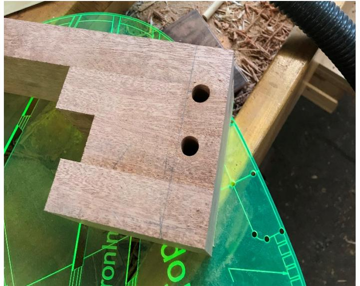
Drill the holes for the KD fitting barrel bolts.
