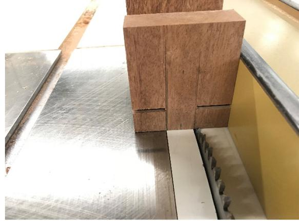
Set the fence to cut just outside the pencil line of the mortise. It's prudent to go well outside the line and "sneak" up on the final cuts.
