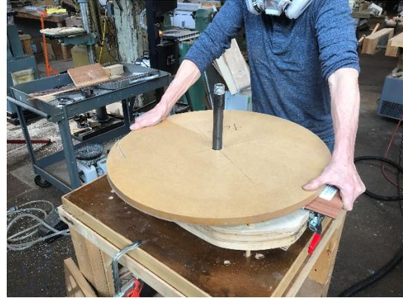
When the chalk marks are gone, you will now put the initial angle on the top bout for the fingerboard extension. Put a 1/8" thick shim at the tail block end between the sides and the radius dish and hold it with one hand as the other hand turns the dish bearing down on the neck block end.
