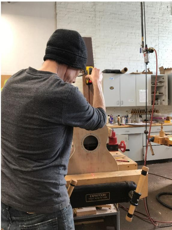
With the neck in the mortise, check with a laser or straight-edge. Use the truss channel center and the body center-lines as reference.
