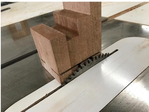
For the final cuts, set the blade just under the cheek cut.
