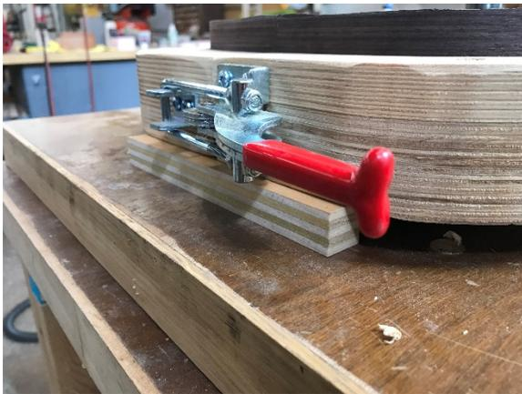
Raise the mold up using  $\frac{3}{4}$ " plywood blocks, one at each end.
