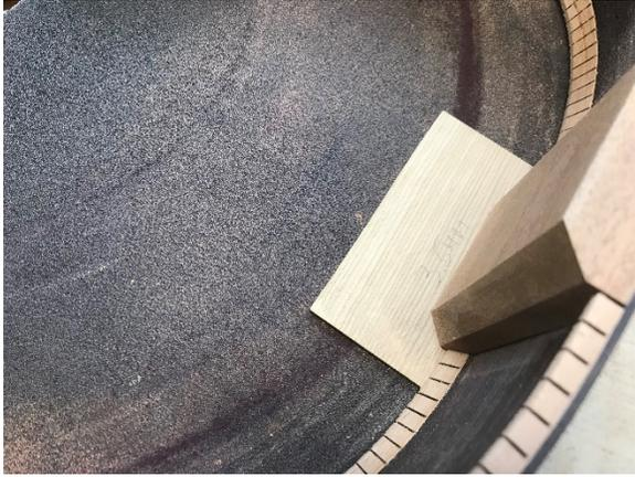
Turn the mold over and with the top now resting on a FLAT sanding dish, put a 1/8" (3.5mm) shim under the tail block.
