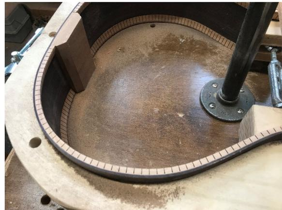
Profile with the dish until the chalk is gone. You really only need to profile the top at this point from the tail block end to about 3-4" from the neck-block.
