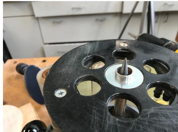
To make sure the mortise is centered front to back, I made a  $\frac{1}{2}$ ' metal scribing bit for my router.
