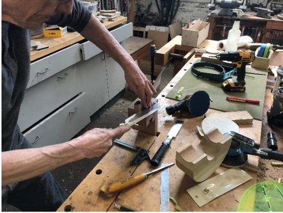
And cut off the excess. Note how I'm pushing down on the saw blade to get it to cut flush. It's OK though if you don't, it's covered up by the heel-cap. Check the final fit in the mortise and adjust if necessary with a shoulder plane.
