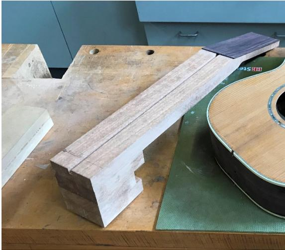
Notes - The truss rod channel is one of the two most important centerlines in my builds. I used to cut it with a router, but I got inconsistent results. Now, I cut it on a table saw using a dado blade. Using a blade that's just under  $\frac{1}{4}$ " wide (the width of my truss rods) I run it down the center of the 3" wide neck blank, then run it down the other side. This centers the channel perfectly in the neck blank. Then I'll attach the peg-head overlay and stacked heel.
