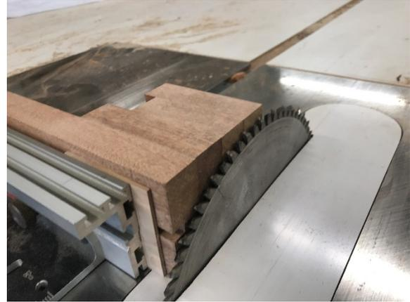
Raise the saw blade as high as it will go. (Note mine does not go up to 3") And cut a small amount of the end off – leaving 7/8" past the mark for the 14<sup>th</sup> fret. Make sure you use a cross-cut blade, not a rip blade. A good combo blade works as well.
