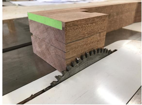
Layout the tenon lines using the truss rod channel as a reference point (that's the reason it must be perfectly centered). Don't raise the sawblade past the line, make it just under.
