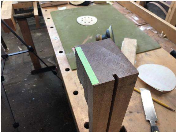
I put a piece of tape there to compensate – the cut MUST be squared perfectly for the next step of cutting the tenon.
