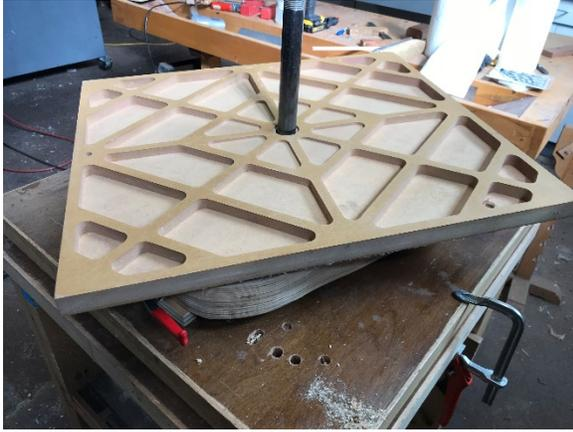
Put the radius on the back – I'm using a standard 15' dish. It should only take a few minutes to remove the chalk.
