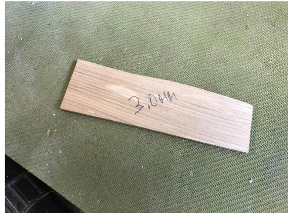
To calculate the neck angle, you will have to use a shim at the bridge location. In Robbie O'Brien's course he uses a 3.5mm shim. I like a lower saddle in the bridge, so I use a 3.0mm
