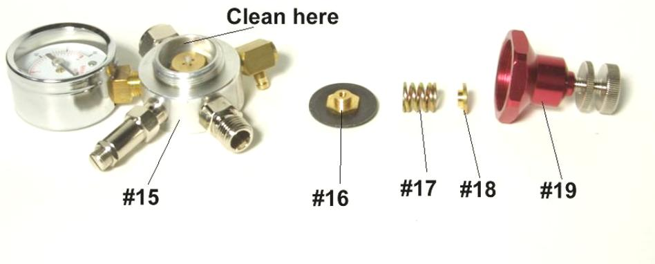
Remove the red housing #19 with a wrench or pliers. Take out parts #18, #17, and #16 from the housing #15. Clean the inside of the housing with a Q tip or small piece of clean cloth. Re-assemble in the order as shown in the above picture. The hex nut at the top of #16 diaphragm seats into the left side of spring #17 when re-assembled. Individual parts to the regulator are not available. If damaged, purchase Part # QS 32-15.
