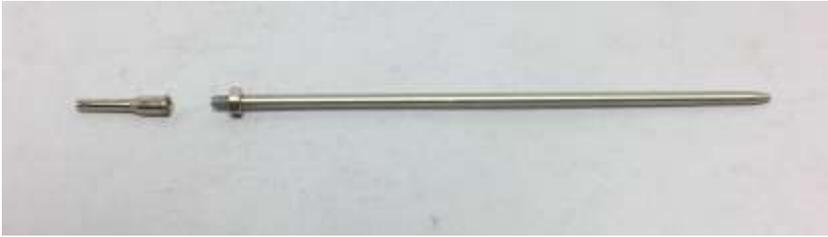
QualSpray needles are made in two parts, separated by the little hex nut towards the back. The length of the needle is set by the factory and should not need adjustment; however it can be adjusted if necessary. This procedure is **ONLY** recommended if there are problems triggering the gun. Improper needle length causes the following issues:
