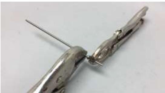
The factory locks the position of the needle with Loctite. Heating the shaft for a bit using a heat gun helps. Using 2 channel locks, grasp the back shaft and the front shaft near the hex nut (see photo). You can then turn the needle to lengthen it. To shorten it, adjust the hex screw towards the back of the shaft. We recommend locking the needle when you are satisfied with the length with Loctite (medium strength)
