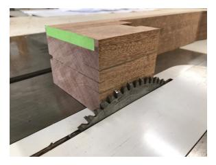
Layout the tenon lines using the truss rod channel as a reference point (that's the reason it must be perfectly centered). Don't raise the sawblade past the line, make it just under.
