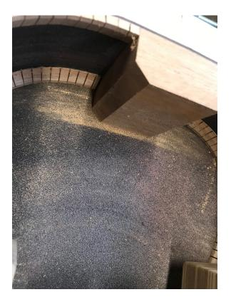
Holding the mold at the tail block end, push the neck block end and start to sand. At first you will see action at the neck block.
