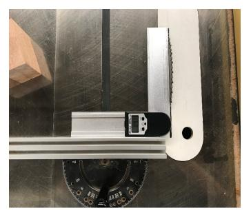
Transfer the angle you measured earlier for the neck (in this case 89.7 degrees) to the miter gauge for your table saw.
