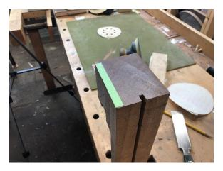
I put a piece of tape there to compensate – the cut MUST be squared perfectly for the next step of cutting the tenon.
