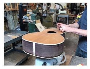
Also scrape or sand the area where the fingerboard extension will lay.
