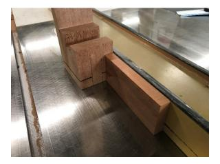
When you do these final two cuts, use a piece of wood that's thinner than the cut to keep the piece from kicking back.
