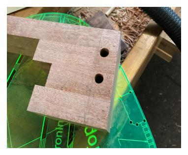
Drill the holes for the KD fitting barrel bolts.
