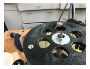
To make sure the mortise is centered front to back, I made a  $\frac{1}{2}$  metal scribing bit for my router.
