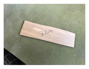
To calculate the neck angle, you will have to use a shim at the bridge location. In Robbie O'Brien's course he uses a 3.5mm shim. I like a lower saddle in the bridge, so I use a 3.0mm
