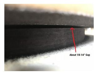
Take the shim out and press down on the dish at the tail block end. You want to see a gap at the neck block end of about 1/8" to 1/4". Don't fuss the measurement too much, you'll do the final profiling after the kerfing, head and tail blocks are installed.
