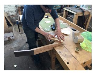
To prepare for cutting the tenon, make sure the neck blank is flush with the stacked heel.
