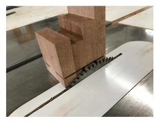
For the final cuts, set the blade just under the cheek cut.
