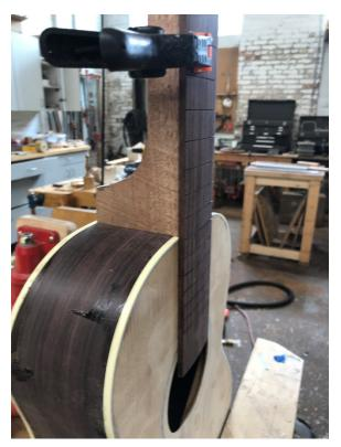
Go ahead and do the rough taper and heel sculpting. Then clamp your fingerboard to the neck and check the fit. This is the result after no flossing or tweaks!!!!
