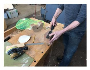
Remove the piece that's left with a flush cut saw.
