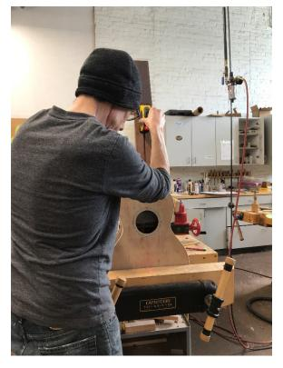
With the neck in the mortise, check with a laser or straight-edge. Use the truss channel center and the body center-lines as reference.
