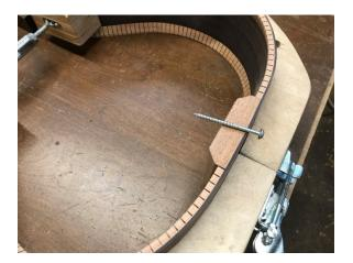
With body top down in the mold, put the ¾" plywood spacers (see pre-profiling) and press down firmly so the top is flat on the table. Make sure all the stretchers are in place. Using 3" wood screws, screw the body to the mold at the neck block and tail block. Make sure the screws don't go through the blocks. You will not remove the body from the mold now until after the top and back are glued on.
