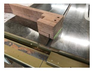
Holding the end of the heel firmly against the fence, cut one cheek.
