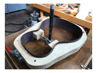
I use acrylic templates (Waldron) to lay-out the side profile and add 5mm. After bending and cutting to length, put them in the mold, top side down. Put in the stretchers.
