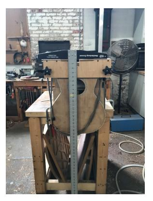
I use Robbie's neck jig to cut the mortise. However, I made some slight changes to the procedure and the jig. First, I get better contact with the body top by using bungee cords to pull the body up. I also use a T-square to make sure the body is in the jig on the centerline of the body.
