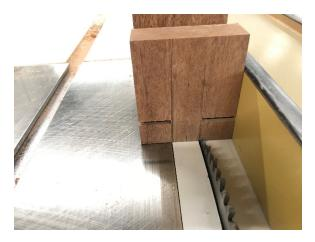
Set the fence to cut just outside the pencil line of the mortise. It's prudent to go well outside the line and "sneak" up on the final cuts.
