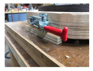
Raise the mold up using  $\frac{3}{4}$ " plywood blocks, one at each end.
