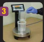
Remove liner from wall dispenser and place in 3MTM PPS™ mixing cup.
