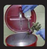
A squeeze bottle (Part No. 37720) containing solvent or water enables fast gun cleaning when the 3M™ PPS™ cup is removed. This means that the operator can switch, for instance, from Basecoat color to Clearcoat without leaving the booth.
