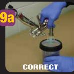
Make sure that the lid fingers are fully engaged above adapter edge.
