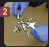
Thread correct adapter into spray gun.
