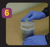
Take a lid (with built-in filter) from wall dispenser and snap onto top of 3M<sup>TM</sup> PPS<sup>TM</sup> cup/liner.
