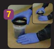
Position locking collar onto the 3M<sup>™</sup> PPS<sup>™</sup> cup/liner and turn until tight.
