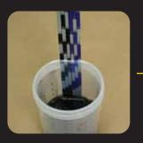
If you are refilling the cup when there is already material in it, and you are not putting it on a scale, put the stir stick at the top of the fluid line to mark your place, and then fill the cup.
