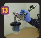
Disconnect air line, invert gun and pull trigger (full open, not partial) to return mix to gun cup before disconnecting gun.
