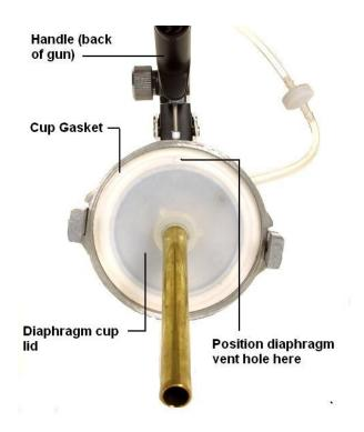
Fill the cup (#3) 3/4 with solvent. For oil based use, spray some mineral spirits, naphtha or lacquer thinner through the gun. For water base, spray water through the gun before using. Install a female 1/4" quick connect that matches your quick coupler of your air hose to the air inlet (#7) of
