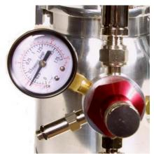
about 5 psi from our test (see photo left) but you can increase the pressure by turning it clockwise. You should operate at 5 psi for most finishes. Increase it for latex or other thick finishes. The higher the psi, the faster the finish will come out of the gun.
