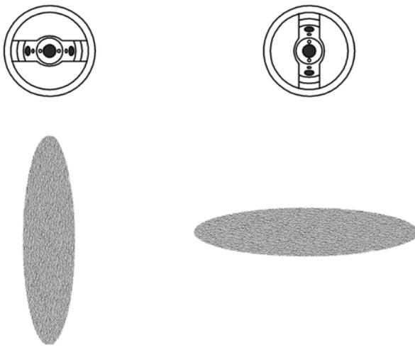
A) Loosen the collar 6094. Turn the air cap 6093 to the horizontal position then re-tighten to collar to lock it into place. This setting produces a vertical spray pattern. This pattern is used more than any other by experienced spray painters.
