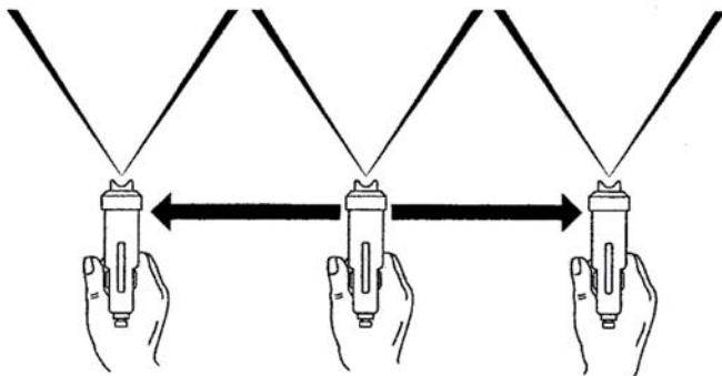
Start moving the spraygun in the direction you want to spray and press the trigger. Between each successive pass, overlap by about a quarter.
