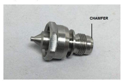
The fluid nozzle has a chamfer on the back of the nozzle. This has to be seated firmly to the fluid passage inside the spray gun. If it isn't one of the following problems will happen
