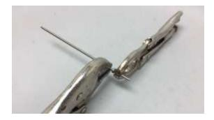
The factory locks the position of the needle with Loctite. Heating the shaft for a bit using a heat gun helps. Using 2 channel locks, grasp the back shaft and the front shaft near the hex nut (see photo). You can then turn the needle to lengthen it. To shorten it, adjust the hex screw towards the back of the shaft. We recommend locking the needle when you are satisfied with the length with Loctite (medium strength)
