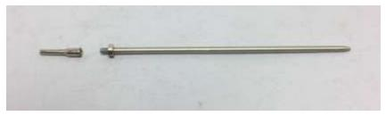
QualSpray needles are made in two parts, separated by the little hex nut towards the back. The length of the needle is set by the factory and should not need adjustment; however it can be adjusted if necessary. This procedure is ONLY recommended if there are problems triggering the gun. Improper needle length causes the following issues:
